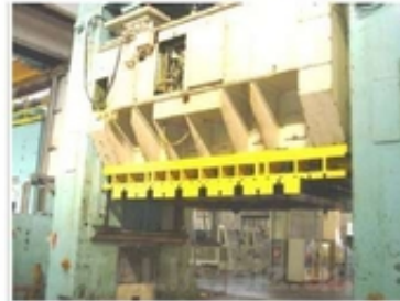
WEINGARTEN ZS 1600.48 MECHANICAL DOUBLE EFFECT DRAWING PRESS
