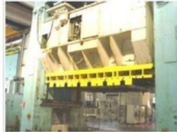
WEINGARTEN ZS 1600.48 MECHANICAL DOUBLE EFFECT DRAWING PRESS
